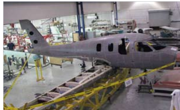
Test fit of wing structure (without top wing skins installed) to fuselage, S/N 002.
